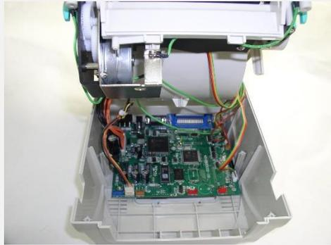
6. Hold the lower cover and lift up the top cover opening levers to separate the lower inner cover from the lower cover.
