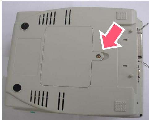
6. Remove the screw that fixes the memory card cover.
