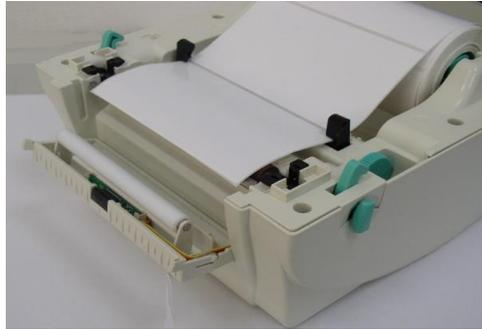
1. Open the peel-off module by pulling it out.
