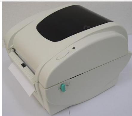
5. Push the peel-off panel back to the printer.
