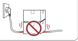
If the product emits a strange sound, burning smell, or smoke, turn off the power immediately and unplug the power cord. If the product is dropped or its exterior is damaged, turn off the power immediately and unplug the power cord. Do not subject the product to shock. **It may start a fire. It may damage the product**.
