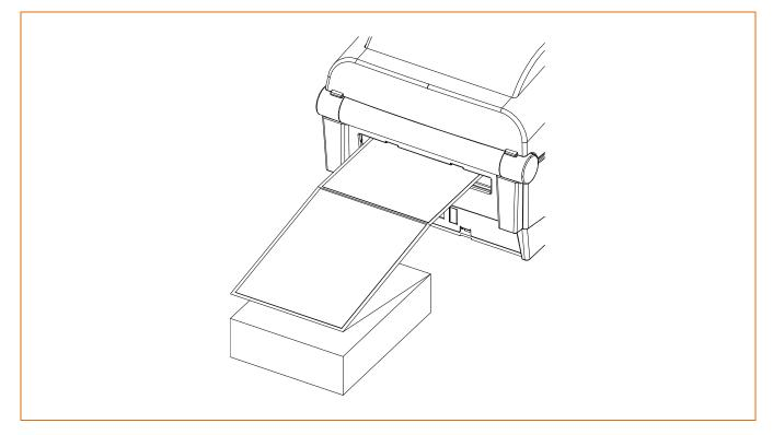
2) Adjust media holders to the media width by using the fix tool.
