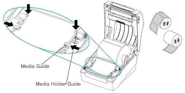
4) After Installation the media, lift the media and manually set the sensor(Black-Mark & Notch Sensor) to the correct position
