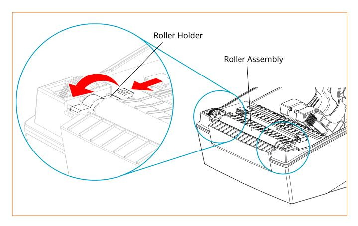
3) Assemble new roller assembly in reverse order.
