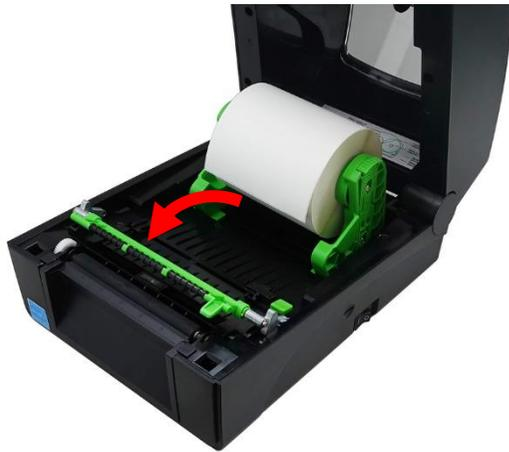
6. Pull the media and thread it through under the media damper until the media extends out of the front panel of the printer.
