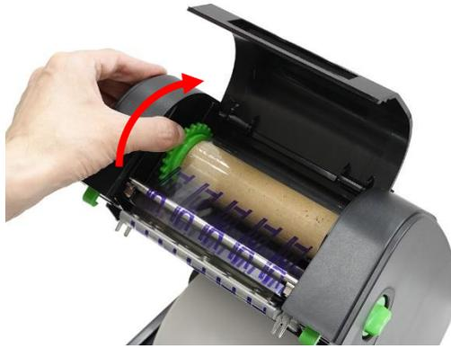
10. Keep rotating the mentioned gear until the ribbon completely covers the printhead and remove any wrinkle from the ribbon.
