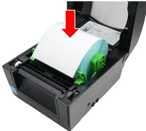
4. Rotate the media to make sure that the media is properly secured and rolls smoothly.
