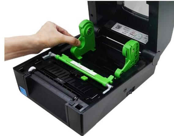
3. Load the media roll into the printer ensuring that the printable side of the media faces up.
