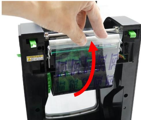
8. Carefully adhere the adhesive strip on the rewind paper core.
