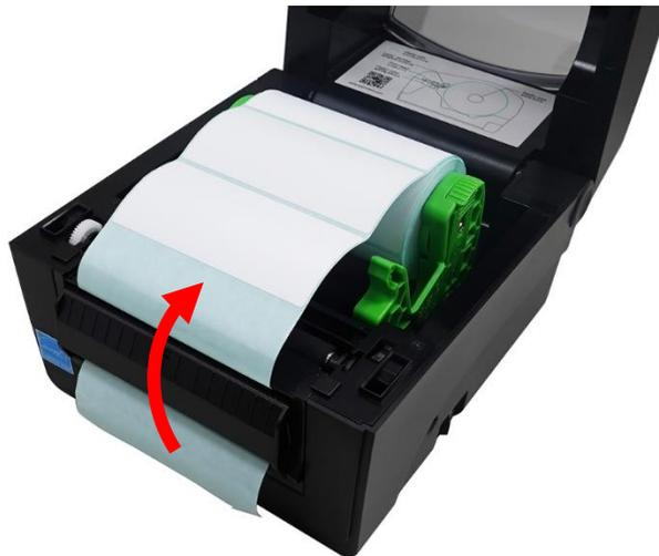
8. Close the printer's top cover. Set the print mode to Peeler Mode and then print a label to check if the peel module works well. For how to set the print mode to Peeler Mode, please refer to 6.7 Configuring Optional Kits and 7.1.1 TSPL.
