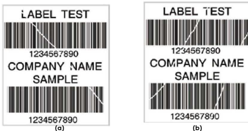
To keep track of the change in print quality, you should adjust the screws by half a turn at a time. Print a test page. If there is no improvement in the print result, turn the screw by another half turn. Do not turn the adjustment screw more than two full turns.
